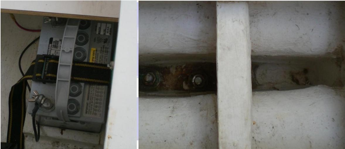
**Figure 4. The picture on the left shows the battery and the picture on the right shows the bilge that is dry. We will inspect the known areas where water collects.**
