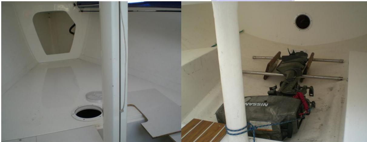
**Figure 2. The two pictures above show the interior of a J80 ready to be weighed. The airtight covers are open and the cover to the battery box is open. The stairs do not have to be attached in their normal location but on board. Water tends to collect in the small forward compartment in the left photo and in the airtight compartments.**
